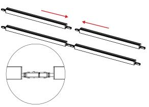
3 Slide the quick connect plugs into the fixture.
