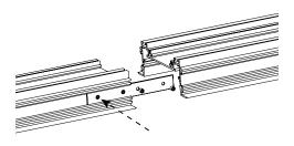
Pull the fixtures together and tighten the remaining screws. Repeat steps for the other side of the fixture.
