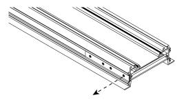
Center the bracket between the 2 fixtures. Secure one side of the joiner to the fixture housing.
