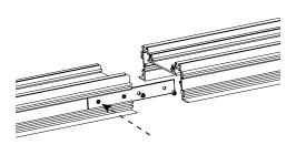
Pull the fixtures together and tighten the remaining screws. Repeat steps for the other side of the fixture.
