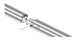
Pull the fixtures together and tighten the remaining screws.
