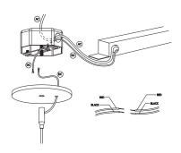
Fasten the MIDDLE OF RUN (MOR) fixture to the EOR fixture by engaging it into the Joiner Bracket. Lightly engage (1) Set Screw if needed. Secure the Power End of the fixture to the ceiling (Ref Step 2). Tighten the Set Screws in the joiner.
